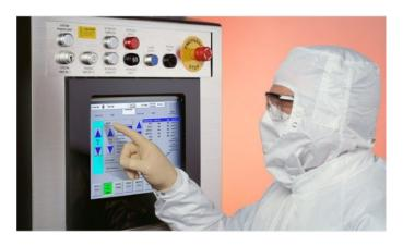
Upgraded PLC control system with Windows OS touch screen GUI. Now offering SECS / GEM interface.
