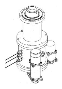
Each Rotation Assembly is completely disassembled and refurbished at the THERMCO-EPITAXY factory.
